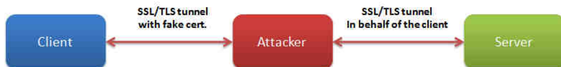
Fig. 1: Structure of a Man In The Middle attack
